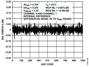
Figure 9. Typical ADC DNL, Differential Mode
