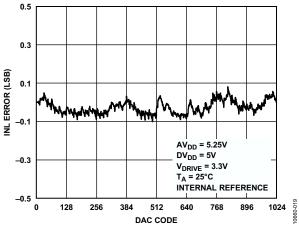
Figure 17. Typical DAC INL vs. Output Code
