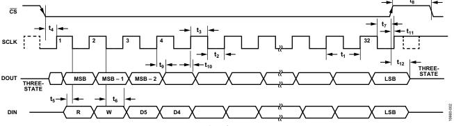
Figure 2. Serial Interface Timing Diagram
