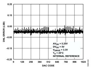
Figure 20. Typical DAC DNL vs. Output Code
