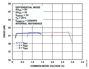
Figure 33. Common-Mode Voltage (Dependent on Input Range)
