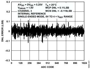
Figure 6. Typical ADC DNL, Single-Ended Mode
