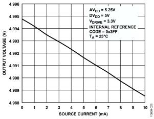
Figure 23. DAC Source Current (Full Scale)
