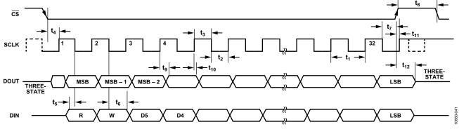
Figure 35. Serial Interface Timing Diagram
