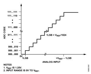
Figure 34. Straight Binary Transfer Characteristic Corresponding to Single-Ended Input Range of 0 V to V<sub>RFF</sub>
