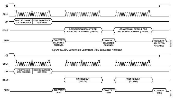
Figure 41. ADC Conversion Command (ADC Sequencer Used)
