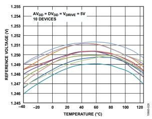
Figure 27. Reference Voltage vs. Temperature
