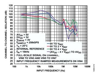
Figure 15. ADC Channel-to-Channel Isolation
