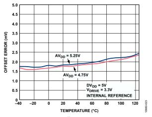
Figure 22. DAC Offset Error vs. Temperature
