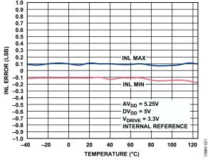
Figure 18. DAC INL vs. Temperature
