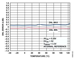
Figure 21. DAC DNL vs. Temperature
