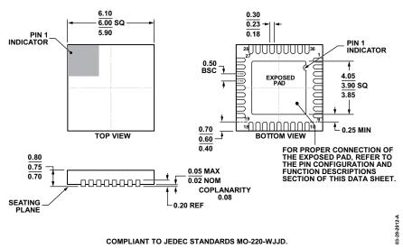
Figure 47. 36-Lead Lead Frame Chip Scale Package [LFCSP\_WQ] 6 mm × 6 mm Body, Very Very Thin Quad (CP-36-3) Dimensions shown in millimeters
