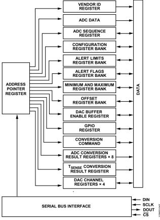
Figure 39. AD7292 Register Structure
