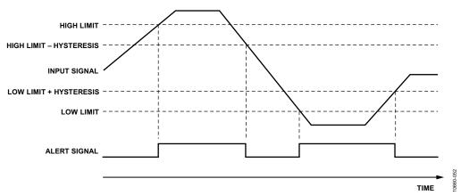
Figure 46. Limit Checking: Alert High Limit, Alert Low Limit, and Hysteresis
