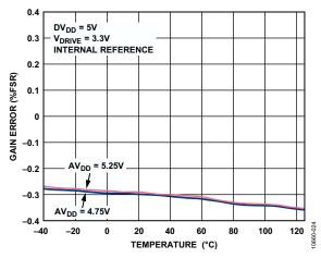
Figure 25. DAC Gain Error vs. Temperature
