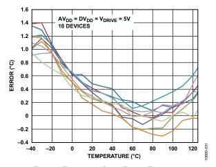
Figure 28. Temperature Sensor Error vs. Temperature
