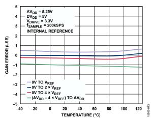
Figure 14. ADC Gain Error vs. Temperature, Single-Ended and Differential Modes
