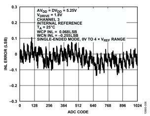
Figure 5. Typical ADC INL, Single-Ended Mode
