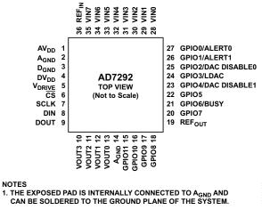
Figure 3. Pin Configuration
