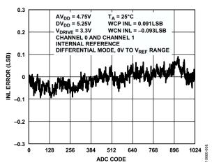
Figure 8. Typical ADC INL, Differential Mode
