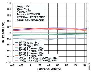
Figure 10. ADC INL vs. Temperature
