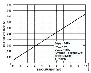
Figure 26. DAC Sink Current (Zero Scale)
