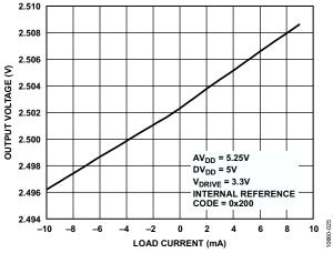
Figure 24. DAC Output Voltage vs. Load Current (Midscale)
