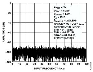
Figure 7. ADC FFT, 200 kSPS,  $f_{IN} = 10$  kHz, Differential Mode
