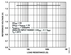
Figure 19. Reference Voltage vs. Load Resistance
